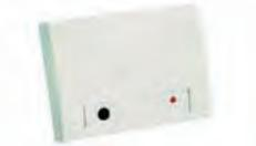
The addressable wireless ShatterPro glassbreak sensor features Pattern Recognition Technology for superior detection and false alarm immunity. It protects all glass types up to a thickness of 1/4 in. Senses through light blinds and drapes. It has a range of 20 ft. and can be wall or ceiling mounted.
