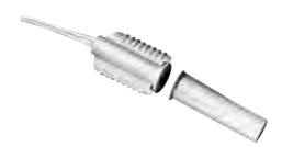
The GE 3/8 in. dia. recessed wing fit magnetic contact is ideal for new construction applications, where wood swell poses a potential threat to the contact housing. The "wings" flex to hold the contact securely in place as the wood expands and contracts.
