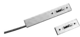
The GE Sensors and Detectors' Maxi-Gap Magnetic Contact is designed for loose or poor fitting overhead doors. The contact helps prevent or correct false alarm situations created by doors that do not line up properly, sag, or that are loose and move with wind or vibration. The channel-mount unit is equipped with the unique Maxi-Gap feature that allows a vertical gap distance of 6 in. and an overall side-to-side gap of 6 in.
