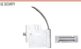
The 2302 Curtain Door Magnetic Contacts are designed specifically for curtain style overhead doors. The unique design allows the contact to be mounted directly to the channel of the door, with the magnet mounted horizontally in the door slats, off the floor and out of harm's way. The interlocking mounting bracket adjusts to fit any size channel width.
