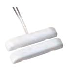
The 1038 Surface-mount Contact is designed for window and door applications where a surface-mount contact is preferred. The switch and magnet are incorporated into the cover housing. Simply mount the base plate using tape or mounting screws (provided), connect the wires and slide the cover housing until it snaps in place.
