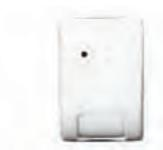
The addressable AP750W PIR motion sensor features Adaptive Signal Processing that analyzes size, speed, shape and adaptive alarm threshold. Provides four separate curtain coverage patterns with 50 ft. range. Flat wall or corner mounting.
