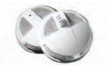
The 400 Series self-diagnostic, four-wire smoke detectors continually monitor their own sensitivity and operational status and provide a visual trouble indication if they drift out of sensitivity range or fail internal diagnostics. They meet NFPA 72 field sensitivity testing requirements without the need for external meters.
