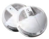
The 400 Series self-diagnostic, two-wire smoke detectors continually monitor their own sensitivity and operational status and provide a visual trouble indication if they drift out of sensitivity range or fail internal diagnostics. They meet NFPA 72 field sensitivity testing requirements without the need for external meters.
