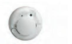
The NX smoke alarm/detector is a Learn Mode wireless sensor that uses photoelectric technology with a self-contained alarm siren, a low battery annunciator, and a status LED. The smoke alarm/detector is part of a security/fire alarm system and communicates with the system control panel.
