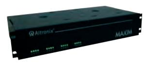
These units distribute and switch power to access control systems and accessories. They convert a 115 V AC input into eight (8) or sixteen (16) independently controlled 12 V DC and/or 24 V DC fuse protected outputs. Outputs are activated by an normally open (NO) or normally closed (NC) dry trigger input from an access control system, card reader, keypad, push button, PIR, etc.
