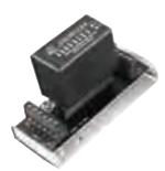
Electrical surges and spikes can render a life saving fire alarm system inoperable. Loop circuits going from building to building are especially vulnerable to voltage surges from storms or electrical faults. Guard critical SLC, IDC and NAC circuits with the 2MHLP series.
