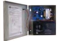
The AL125UL is a power limited power supply/charger that will convert 115 V AC input into two individually PTC protected 12 V DC or 24 V DC outputs. They are intended for use in applications requiring UL listing for access control (UL 294) and applications requiring an interface with Fire Alarm Control Panels (FACP). It must be installed in accordance with national and local electrical codes and regulations.
