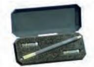
The Corning Cable Systems VFL-350 Visual Fault Locator/Light Source is used to check single-mode and multimode optical fiber cables and components for faults or to locate individual fibers in a bundle. By transmitting a bright beam of red light into a fiber, breaks or improper terminations can be seen as a glowing red light. The VFL-350 emits visible laser light of 635 nm with an output power less than 1 mW. The robust and compact metal housing makes the device suitable for daily on-site use.
