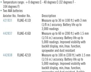
backlit display, min./max. function, spraywater and dust resistant. Audible feedback for taking room angle and incremental measurements, +/- 45 degree tilt for talking indirect measurements in hard-to-reach areas
