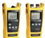
The Corning Cable Systems LTK-400 Series offers a complete, cost-effective solution for link-loss testing of both multimode and single-mode systems for those users who do not require data storage capabilities. The LTK offers unparalleled performance by combining a source that has one of the highest-output powers in the industry with a meter that has 10 calibrated wavelengths. The units can be powered by standard AA alkaline batteries, or by the supplied AC power adapters.
