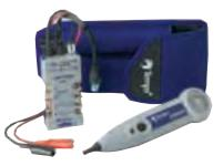
Designed for the network installation and maintenance professional, the LAN Toner sends tone and blinks hub, switch port and PC activity lights for fast identification. This kit can be used on any wiring system including datacom, telecom, security/ alarm, audio and CATV. Kit includes AT8L LAN toner, 200GX inductive amplifier probe and carrying case.
