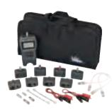
The VDV PRO cable tester is an easy-to-use cable testing and verification device that can quickly test all wiring requirements found throughout today's residential and commercial environments. This tester tests for opens, shorts, split pairs, reversals and miswires on UTP cables, and opens and shorts on coax. It supports RJ11/12, RJ45, coax, F, BNC and RCA connectors. The IENet PRO version supports RJ45 and MJ12 connections and tests to PROFINET industrial Ethernet cabling requirements.
