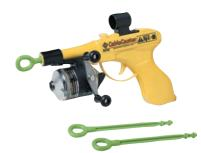
The CableCaster makes installation of cable in ceilings, rafters, subfloors and other hard-to-reach areas significantly faster and easier. The CableCaster is a hand-held, dartgun-like device that can fire a dart accurately up to 50 ft. The dart carries a monofilament line from a take-up reel. The communications cable is then attached to the dart and reeled back to the installer.
