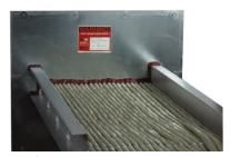
The SpecSeal Composite Sheet is a lightweight, rigid, fire-resistant panel composed of an intumescent layer bonded to a galvanized steel sheet reinforced with steel wire mesh covered with aluminum foil. Reduces large openings and can be combined with other SpecSeal or EZ-Path Firestop products.
