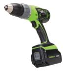
The LHD-216 provides heavy-duty drilling, bit performance and hammer function for drilling up to 1/2 in. holes in masonry and up to 5 in. holes in plywood. It is truly a multi-purpose tool. Turn the chuck collar to any of the 18 clutch positions for bit driving, drilling or hammer drill position. Yet with all of these functions, it only weighs 5.6 pounds.
