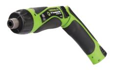
This screwdriver can be used to drive a wide variety of screws and to drill small diameter holes. To fit a variety of situations, it can be used as a straight tool or as a pistol style tool. It has 21 clutch stages to precisely provide the right torque for almost any screw, and when the clutch setting is reached, the tool automatically shuts off to save battery and clutch life.
