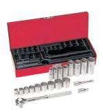
Set consists of 20 pieces: four 6-point sockets, 3/8 in., 7/16 in., 1/2 in. and 9/16 in.; five 12-point sockets, 5/8 in., 11/16 in., 3/4 in., 13/16 in. and 7/8 in.; eight 6-point deep sockets, 3/8 in., 7/16 in., 1/2 in., 9/16 in., 5/8 in., 11/16 in., 3/4 in. and 13/16 in.; two extensions 1 3/4 in. and 3 in. long; ratchet plus metal box.
