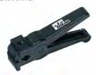
The IDEAL cable stripper has a slide adjustment to accommodate RG-58, RG-59, RG-59/62, RG-8, Belden 8281, Thinnet plenum and twinaxial cable. Two- or three-level strips are available with interchangeable blade cassettes. These blades also can be adjusted individually. Can be used on most standard coaxial cable.
