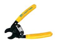
Cuts round communications cable and maintains cable geometry for better cable performance. The Data T-Cutter cuts multipair cable up to 0.5 in. (12.7 mm) and coaxial cable up to RG-9/U. Blade-cutting capabilities are suitable for soft cables (not ACSR).
