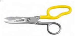
Heavy-duty, nickel-plated, tempered steel scissors with adjustable screw hinge and rounded points. Scissors are 5 in. long with a serrated lower blade. The upper blade includes 19- and 23-gauge wire stripping notches.
