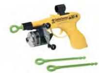
The CableCaster makes installation of cable in ceilings, rafters, subfloors and other hard-to-reach areas significantly faster and easier. The CableCaster is a handheld, dartgun-like device that can fire a dart accurately up to 50 ft. The dart carries a monofilament line from a take-up reel. The communications cable is then attached to the dart and reeled back to the installer.
