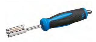
Combines two tools into one: a 7/16 in. hex socket and 3/8 in., 32-threaded end. The hex socket makes installation and removal of CATV F-connectors and CCTV BNC connectors easy. Threaded end holds F-connector during cable insertion to ease connector seating against dielectric and eliminates chance of injury from cable center conductor. Chrome finish for long life, comfort grip.
