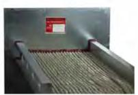
The SpecSeal Composite Sheet is a lightweight, rigid, fire-resistant panel composed of an intumescent layer bonded to a galvanized steel sheet reinforced with steel-wire mesh covered with aluminum foil. Reduces large openings and can be combined with other SpecSeal or EZ-Path Firestop products.
