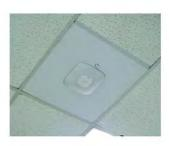
TerraWave's ceiling tile enclosures contain and protect an access point or an antenna system in an aesthetically pleasing and stealthy solution within a suspended ceiling. Suspended in a similar manner as the ceiling tile, they are tethered by wire to the roof structure. Once installed, the AP is protected and hidden from view and the enclosure is flush with the ceiling tile. Every TerraWave enclosure is covered by their two-year warranty program.
