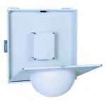
The AAT-ACE-DOME is a ceiling-mount enclosure for wireless access points designed for use in open office spaces. AAT-ACE-DOME replaces a single 2 ft. x 2 ft. drop-ceiling tile. The opaque dome is 14 in. in diameter and projects 6.5 in. below the drop ceiling. The dome is mounted on a fully hinged locking door providing easy access to equipment and cables for authorized technicians only.
