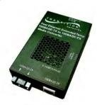
Designed to operate in Fast Ethernet environments where ambient temperatures can rise as high as  $65^{\circ}$ C (149°F). Operating temperature: -25°C to  $+65^{\circ}$ C with 100BASE-TX RJ45 to 100BASE-FX connection.
