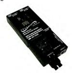
Stand-alone media converters from Transition Networks ship with a 120 V AC power supply. But for those applications where the source of power is DC, Transition offers a variety of wide input stand-alone and piggyback DC power supplies.
