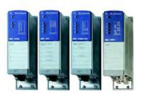
MICE media modules are hot-swappable and may be used with the PowerMICE switch to obtain desired port density. The only restriction is the number of slots that the PowerMICE has (one media module per slot). MICE media modules come a variety of configurations including: copper, fiber (SFP), multimode, single-mode, Gigabit and real-time.
