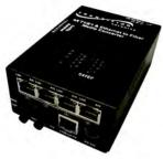
This remotely managed transport MUX media converter can transport up to four T1/E1 lines (RJ48), an RS-232 data channel and a 10/100 Ethernet line over a pair of fiber optic cables. This converter will address the need to conserve installed fiber strands by combining multiple signals and transporting them over one fiber link. Converters supporting single-strand fiber optics are also available.
