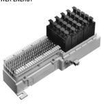
The R66P25QC offers protection for 25 pairs with quick-connect clips for both input and output cable pairs. The unit has the same mounting dimensions as a standard 66M block, and can be mounted on a wall, frame or 89 bracket. Order standard five-pin protector modules separately. One per pair. Requires a 66-termination tool.
