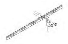
The Multiple Ground Bus Bar allows for the common grounding of multiple Ultron and UltraLinx lightning protectors on the same 66M block and can connect up to 25 protectors (one protector per pair). The bus bar is equivalent to a No. 6 AWG wire and is made of tin-plated copper. The bar is scored on both sides, allowing it to be broken into smaller sections for cost-efficient and customized usage. 10 in. long, 1/2 in. high.
