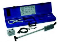
The Tracker II traces the path and determines the depth of wires and metallic pipes on active or dead systems without having to deactivate the system. The transmitter has a distance range of up to 4,000 ft. and depth up to 7 ft. Transmitter output and receiver sensitivity are adjustable.
