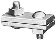
Parallel grooves trap strand tightly without marring. Plate halves align evenly for easy application. Each bolt has a shoulder to prevent turning while tightening.
