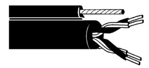
Self-supporting IMREW wire is used for subscriber lines in exchange plant. Single pair is often used for lateral runs from aerial plant. Wire core is laid parallel to a solid steel support wire and jacketed in integral extrusion to form a Figure 8 configuration.
