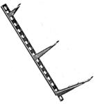
Hot-dip galvanized racks with hook holes  $1\ 1/2$  in. apart. Fasten to manhole or interior walls with 1/2 in. x 4 in. expansion bolts (not included). Mounting slots 5/8 in. x 3/4 in. at top and bottom of 15 in., 24 in. and 30 in. lengths overlap for assembly in combinations for overall length desired.
