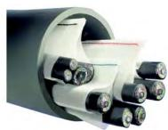
MaxCell is the only flexible, multicelled, textile innerduct specifically designed for the network-construction industry. The unique textile construction allows MaxCell to conform to the shape of cables placed within, greatly reducing the wasted space associated with rigid innerduct. It is available in multiple configurations and lengths.
