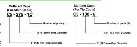
Choose the correct collared and multiple end caps to meet your cable diameter and configuration. (Refer to end cap configurations in the chart.)
