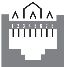
Figure 9a – IEC 60603-7 series interface for Category 5, 6 and 6A. Please note the categories refer to the IEC requirements and not the TIA-568 range of standards.
