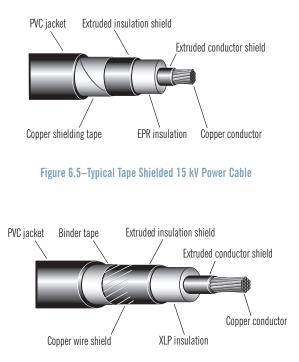
Figure 6.6–Typical Wire Shielded 15 kV Power Cable
