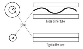
Figure 6.12–Optical Fiber Cable Designs
