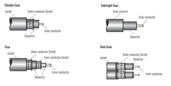
Figure 6.8–Common Types of Coaxial Cable
