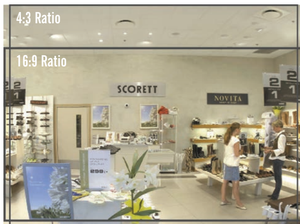
Figure 2 : 16:9 ratio vs. 4:3 ratio Image courtesy of Axis Communications
