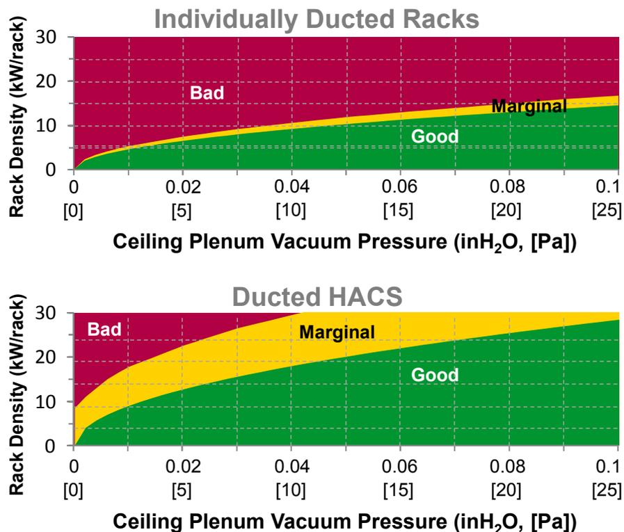
**Figure 8** summarizes the maximum rack density limits of **Figure 7** and facilitates a more direct comparison of performance between ducted racks and ducted HACS. Ideally, ceiling plenum pressure should be maintained at just the values indicated by the curves of **Figure 8** as these are the neutral-pressure operating points for the IT equipment. Lower values of ceiling vacuum result in some hot-exhaust recirculation while higher values imply wasted
