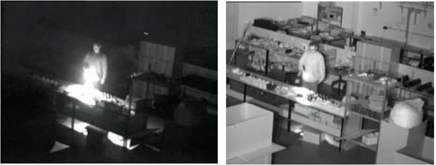
Figure 2.3c At left, image without an IR illuminator; at right, image with an IR illuminator.
