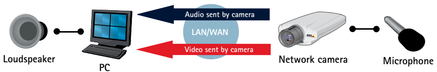
Figure 8.3a In simplex mode, audio is sent in one direction only. In this case, audio is sent by the camera to the operator. Applications include remote monitoring and video surveillance.
