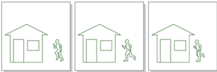
Figure 7.1a With the Motion JPEG format, the three images in the above sequence are coded and sent as separate unique images (I-frames) with no dependencies on each other.
