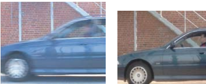
Figure 3.4b At left, a full-sized JPEG image (704x576 pixels) from an analog camera using interlaced scanning. At right, a full-sized JPEG image (640x480 pixels) from an Axis network camera using progressive scan technology. Both cameras used the same type of lens and the speed of the car was the same at 20 km/h (15 mph). The background is clear in both images. However, the driver is clearly visible only in the image using progressive scan technology.
