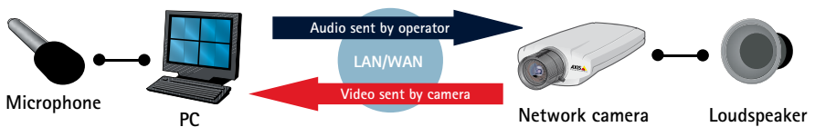
Figure 8.3b In this example of a simplex mode, audio is sent by the operator to the camera. It can be used, for instance, to provide spoken instructions to a person seen on the camera or to scare a potential car thief away from a parking lot.
