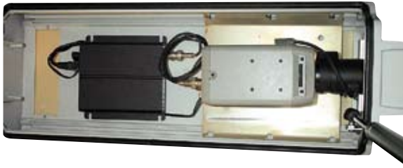
Figure 5.2a An illustration of how a small, single-channel video encoder can be positioned next to an analog camera in a camera housing.
