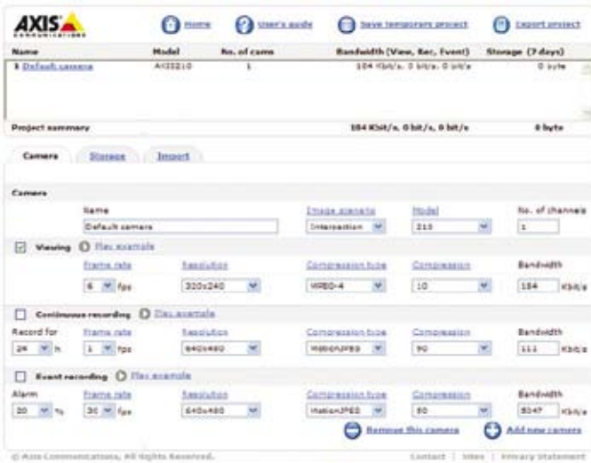
Figure 12.1a The AXIS Design Tool includes advanced project management functionality that enables bandwidth and storage to be calculated for a large and complex system.
