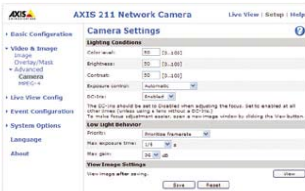
Figure 3.2d A camera user interface with options for setting, among other things, exposure in low-light conditions.
