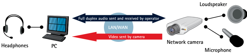
Figure 8.3d In full-duplex mode, audio is sent to and from the operator simultaneously. This mode of communication is similar to a telephone conversation. Full duplex requires that the client PC has a sound card with support for full-duplex audio.
