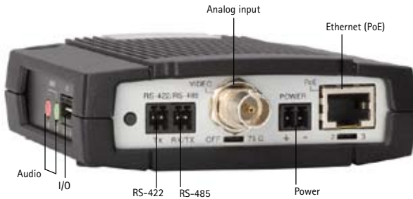
Figure 5.1b A one-channel, standalone video encoder with audio, I/O (input/output) connectors for controlling external devices such as sensors and alarms, serial ports (RS-422/485) for controlling PTZ analog cameras and Ethernet connection with Power over Ethernet support.
