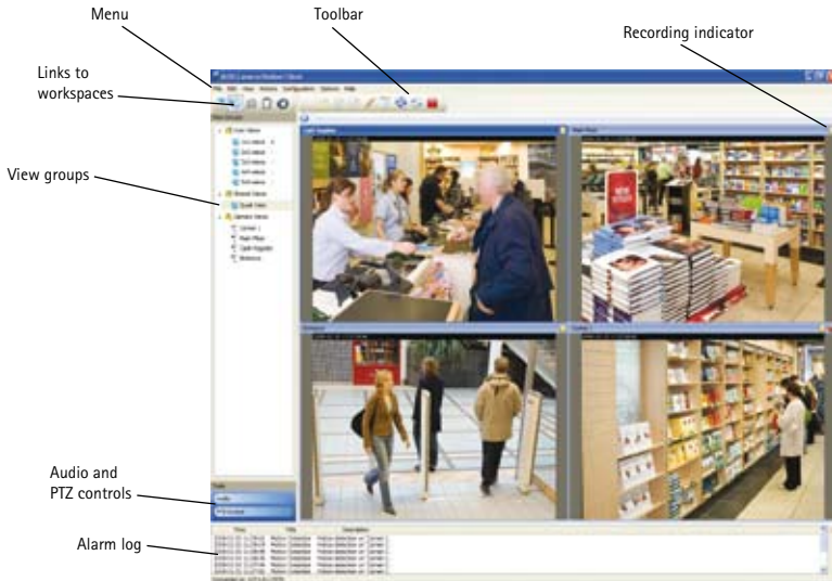
Figure 11.3a AXIS Camera Station's live view screen.
