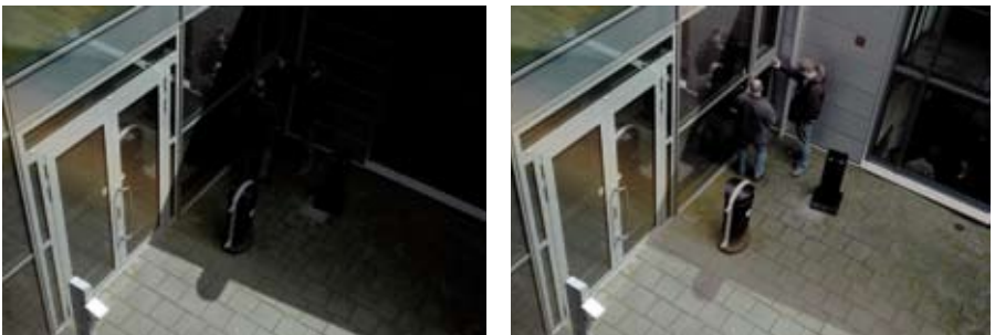
Figure 3.5a At left, image without wide dynamic range. At right, image with wide dynamic range applied.
