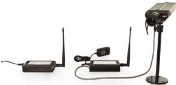
Figure 10b By using a wireless bridge, any network camera can be used in a wireless network.
