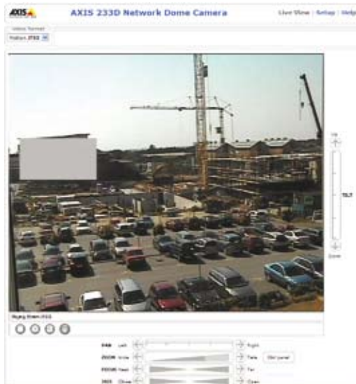
Figure 2.2c With built-in privacy masking (gray rectangle in image), the camera can guarantee privacy for areas that should not be covered by a surveillance application.
