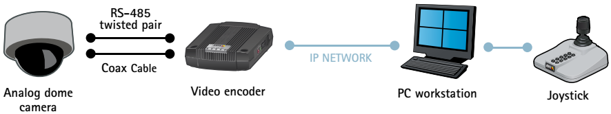
Figure 5.4a An analog PTZ dome camera can be controlled via the video encoder's serial port (e.g., RS-485), making it possible to remotely control it over an IP network.
