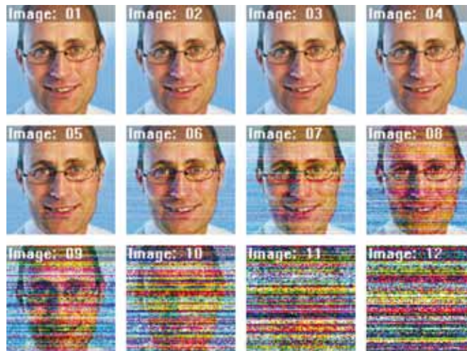
Figure 8: Subject taken from a standard camera with unchanged settings. Subject is moved into darker and darker shade, resulting in increased noise.
