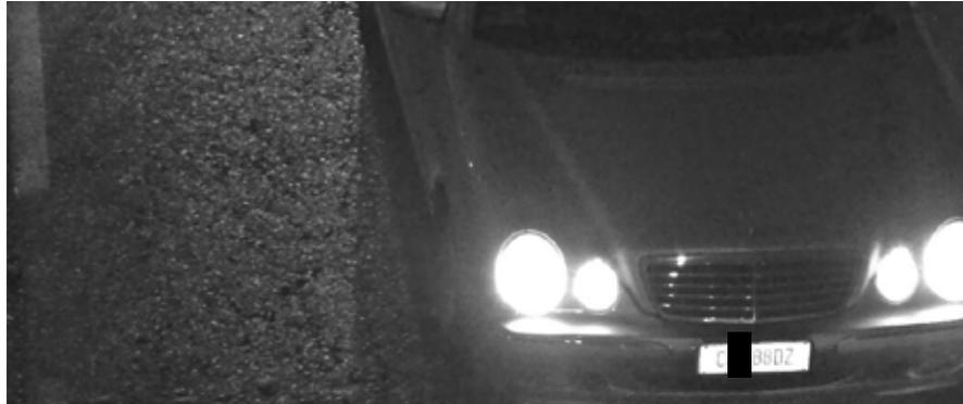
Figure 3: IR illumination used for license plate recognition (LPR)
