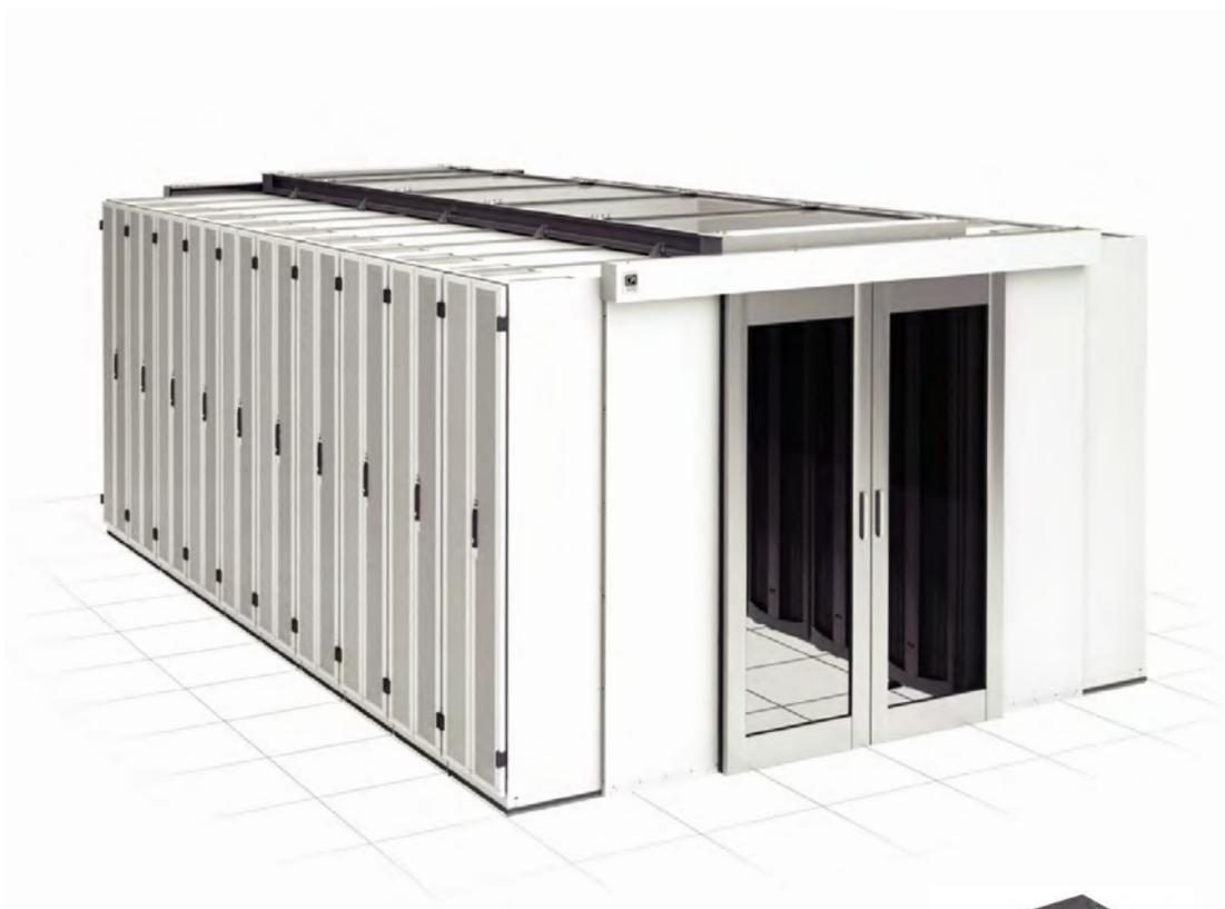
In this example, CPI Aisle Containment Doors are combined with a Cabinet Supported Ceiling Panel Kit and the F-Series TeraFrame® Cabinet System to enclose the cold aisle between adjacent cabinet rows. The overhead ceiling traps cold air in the aisle so that it will be used to cool equipment, instead of the entire room.
