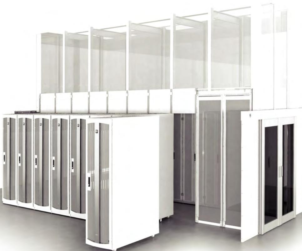
In this example, CPI's Aisle Containment Doors are combined with the F-Series TeraFrame® Cabinet System and a Frame Supported Exhaust Duct to enclose the hot aisle between adjacent cabinet rows. While CPI cabinets are used in this example, the Frame Supported HAC is also compatible with other cabinet brands. This example also shows how the overhead duct extends toward the ceiling, ensuring that all hot exhaust air is completely isolated from the rest of the room.
