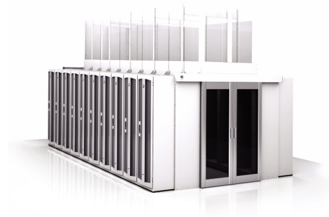
Figure 6: Standard Hot Aisle Containment Solution by CPI. In the example above, CPI's Aisle Containment Doors are combined with the F-Series TeraFrame® Cabinet System and an overhead duct to enclose the hot aisle between adjacent cabinet rows and the overhead duct is used to isolate hot exhaust air from the room.
