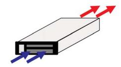
Figure 3 – Typical server airflow
