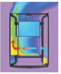
Figure 6 – Re-directing exhaust out rear of cabinet
