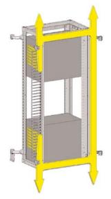
Figure 8 – Cable routing inside cabinet
