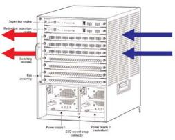
Figure 4 – Cisco switch side-to-side airflow
