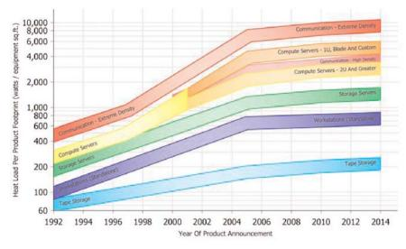
Source: Datacom Equipment Power Trends and Cooling Applications" ©2005 American Society of Heating, Refrigerating and Air-Conditioning Engineers, Inc.
