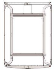
Figure 5 – Offset bracket creating recessed frame design
