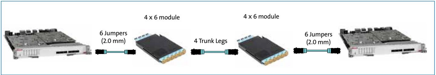
The harness-based design for Pretium EDGE® AO Solutions uses standard MTP® Panels that connect to preterminated conversion harnesses. Like the conversion modules, Pretium EDGE AO Conversion Harnesses enable the greatest fiber utilization from the base-12 backbone trunks by converting from 12-fiber MTP connectivity to 8-fiber MTP connectivity. The 8-fiber MTPs of the harness then connect to the electronics via MTP jumpers.
