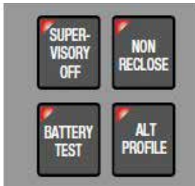
Figure 13. One-touch function keys.
