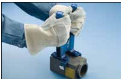
Fig. 9 If the mold does not seal properly, make adjustments to the handle clamp.
