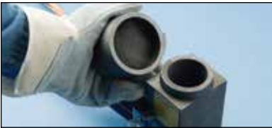
Fig. 27 Remove the alligator clips from the igniter pin. Remove the graphite cover of the ERICO CADWELD EXOLON mold.
