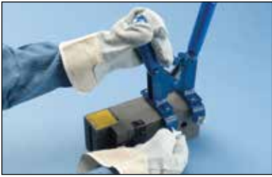
Fig. 7 Tighten the clamp thumbscrews onto the mold.
