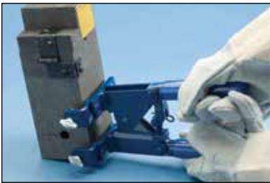
Fig. 8 Close the grips to tightly lock the mold. Check for an appropriate seal on the mold.
