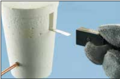
Fig. 12 Place the ignition strip into the control unit connector. Remove or protect fire hazards in close proximity to the connection. Advise nearby personnel of welding operations in the area.
