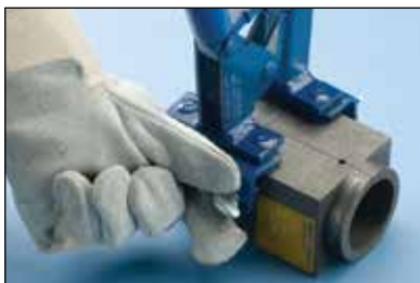
Fig. 7 Tighten the clamp thumbscrews onto the mold.
