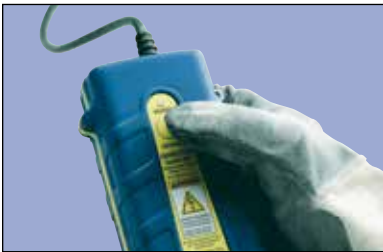
Fig. 13 Using the control unit, press the button and hold, while you observe the "ready" indicator light. A green light will blink for a few seconds and then will change to a constant light. At this time, the unit will send a charge to the ignition strip. The ignition strip will spark inside the metal cup, activating the ERICO CADWELD PLUS exothermic reaction.
