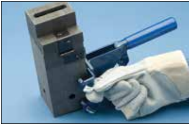
Fig. 7 Tighten the clamp thumbscrews onto the mold.
