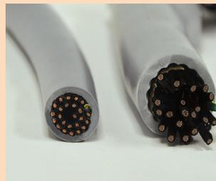
**Swelling** – Caused during exposure of the PVC to oil or other chemicals due to migration of the oils into the plasticizer, resulting in noticeable increases in insulation and jacket diameter.
