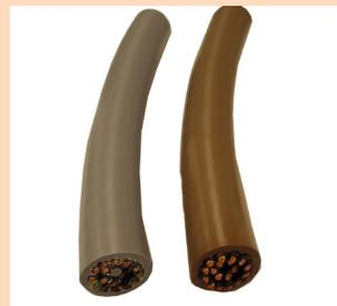
**Discoloring** – Caused during the exposure of the PVC to oil or other chemicals due to the diffusion of the plasticizers along with colorant from the insulation and jacket.
