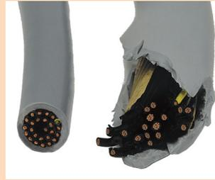
**Cracking** – Caused during exposure of the PVC to oil or other chemicals due to the complete removal of plasticizers, resulting in hardening and eventual cracking of the insulation and jacket.
