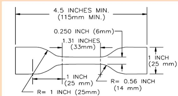
Untested die cut samples are aged under the UL Oil Res II requirement of 75°C for 60 days. After 60 days, the samples are removed from the oil for a minimum of 16 hours. They are then tested for tensile and elongation, which must retain 65% of the unaged values. The following is an example for an Oil Res II test results:
