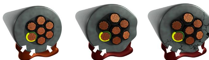
*Oil can cause polymers, such as those used for cable insulation and jacketing, to degrade and crack. Selecting an oil-resistant cable is the best way to avoid this failure mode.*
