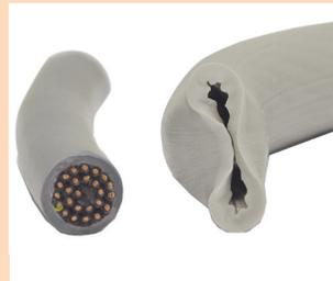
**Melting** – Caused during exposure of the PVC to oil or other chemicals due to the absorption and combination with the plasticizer, resulting in softening and the high elasticity noted in the compound.
