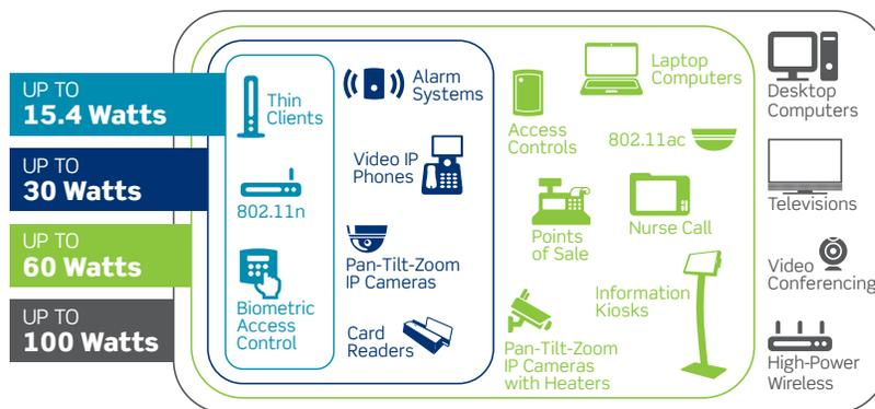
Both PoE tiers under the 802.3bt standard will support a range of enterprise devices, such as laptops and desktop computers, exterior-mounted IP cameras, information kiosks, industrial automation equipment, and next-generation wireless access points (WAPs). Publication of 802.3bt is anticipated for Q4 of 2018.
