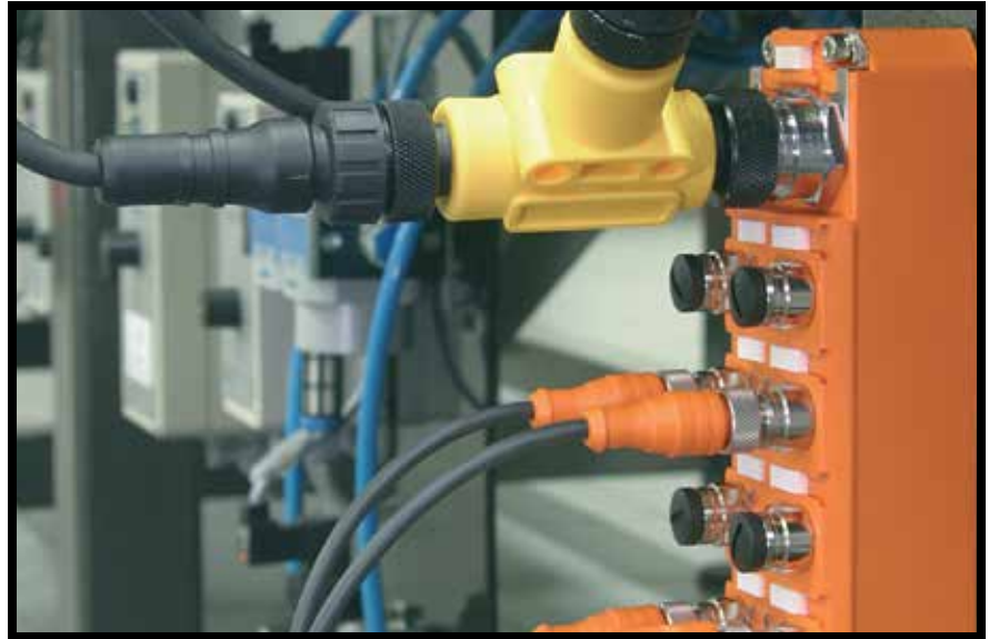
Using a simple cabling architecture to connect modules is much easier than redesigning a centralized cabling system each time, and the resulting modules cost less to build and deploy.
