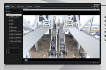
Integrated devices and other connected systems can be controlled directly with overlay buttons from the camera view, streamlining workflows and improving operator efficiency.
