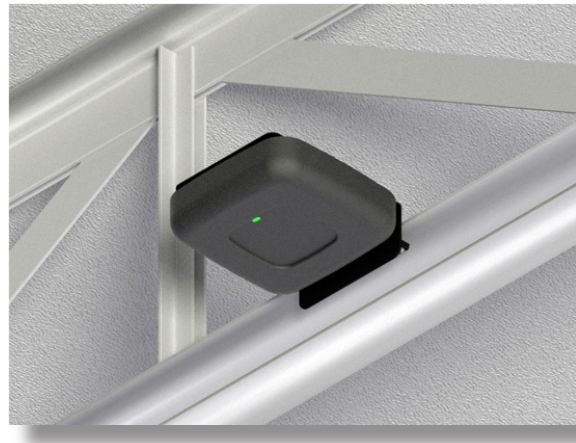
Model 1006-CCOAP (left) Right angle brackets are designed to mount leading vendors' APs in the preferred orientation. Model 1008 (Right) right angle bracket includes a paintable vanity cover to conceal APs in open "red iron" ceilings
