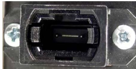
MPO adapter shown with connector installed inside the cassette
