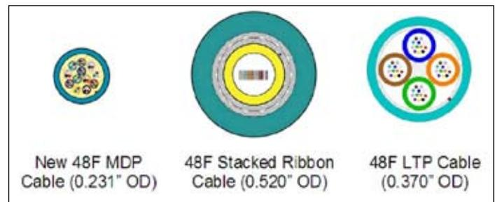
Figure 1. Reduced-diameter cables save space in crowded conduits.
