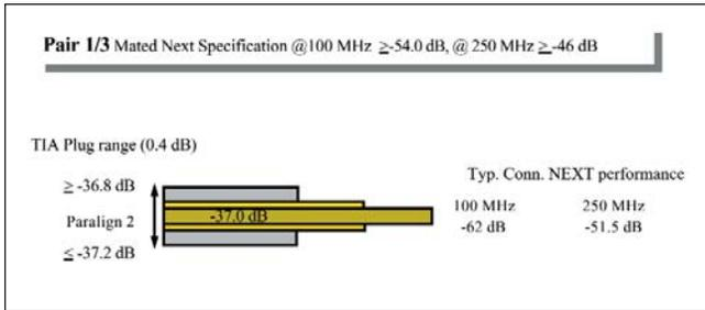
Testing at higher frequencies (250 MHz) re-enforces the benefits of center tuning. NEXT values for positions 3, 4, 5 and 6 of the mated union of the centered connector and the 36.4dB plug termination were 47.5dB. For the mated union of the centered connector and the 37.6dB plug termination, the NEXT values were 48.0dB. Lastly, for the mated union of the centered connector and the centered plug termination of 37dB, the NEXT value was 51.5dB.
