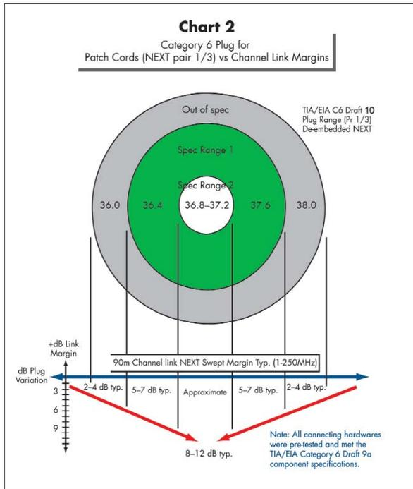
designed to these targets. It does no good to have jack and panel ports with different values since both need to connect with the same patch cord design. In fact, the patch cord terminated plug value should be the foundation value to which all other connectivity is built.
