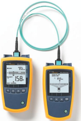
Figure 4. MultiFiber™ Pro power meter and light source.
