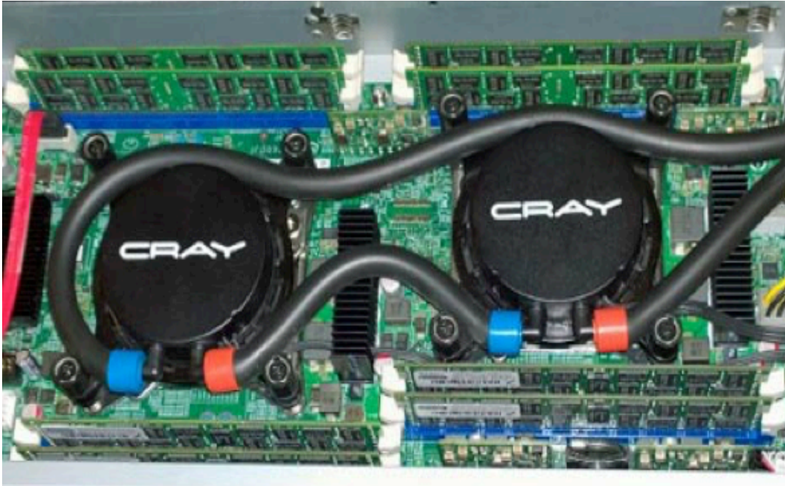
Figure 8- A look at server for a Cray CS400 supercomputing cluster, which is cooled with an Asetek system that brings warm water to the chip. (Photo: Rich Miller)
