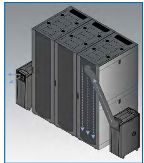
Portable air conditioning units can direct cold air through directional louvers or a flexible output duct.
