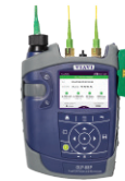
SmartClass Fiber OLP-88 PON power-level measurement, GPON ONT activation process verification, ONT/ONU identification, rogue/alien-ONU detection, and connector inspection with pass/fail analysis
