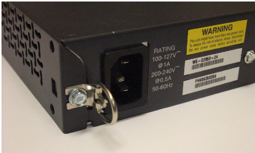
Figure 2 – Example Installation of Tie Wrap Retainer
