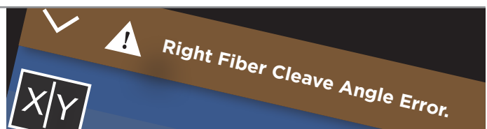
Figure 1. According to SumiCloud™ splice data, approximately 15% of fiber preparations are rejected by the splicer because of poor cleaves.
