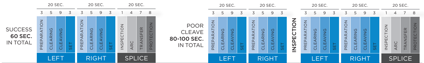
Figure 3. Time chart comparison between (a) a successful splice vs (b) rework due to poor cleaves (The time was measured using a single fiber core alignment splicer. Time for each process may vary depending on the skill of operators.)
