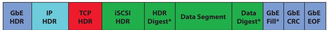
Figure 1: Shown are the several layers make up an iSCSI packet. Transactions begin with just the iSCSI portion (in green) and build out through TCP (red), IP (light blue), and Gigabit Ethernet (dark blue). While the TCP checksum and Gigabit Ethernet CRC can detect some bit errors in iSCSI headers and payloads, they do not detect errors generated at iSCSI protocol crossovers.
