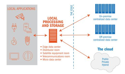
**Edge computing** describes a data center topology in which information processing and content collection and delivery are placed closer to the sources of this information. The goals are to reduce latency, reduce unnecessary traffic and establish a hub for interconnection between interested peers and for data thinning of complex media types or computational loads.<sup>4</sup>
