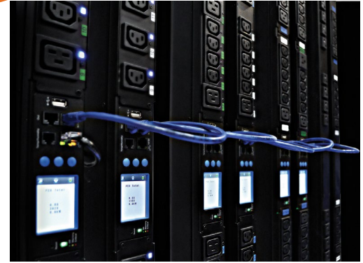
IP consolidation - links up to 20 PDUs under a single IP address
