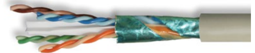
Uniquely designed isolation wrap contains discontinuous sections of metalized material, held in place by a polymeric layer.
