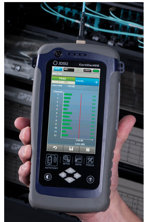
View test set up and results data and edit labels at both local and remote ends.
