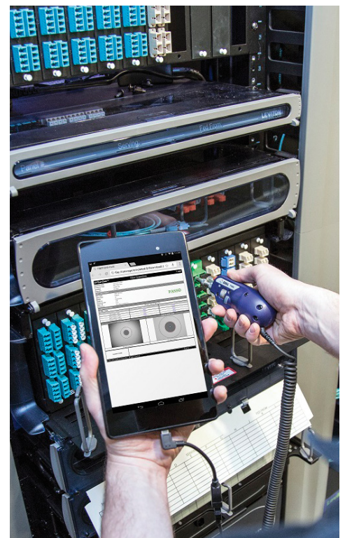
Easily connect to mobile Android™ devices/tablets using FiberChekMOBILE.
