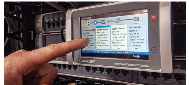
imVision controller showing circuit trace
