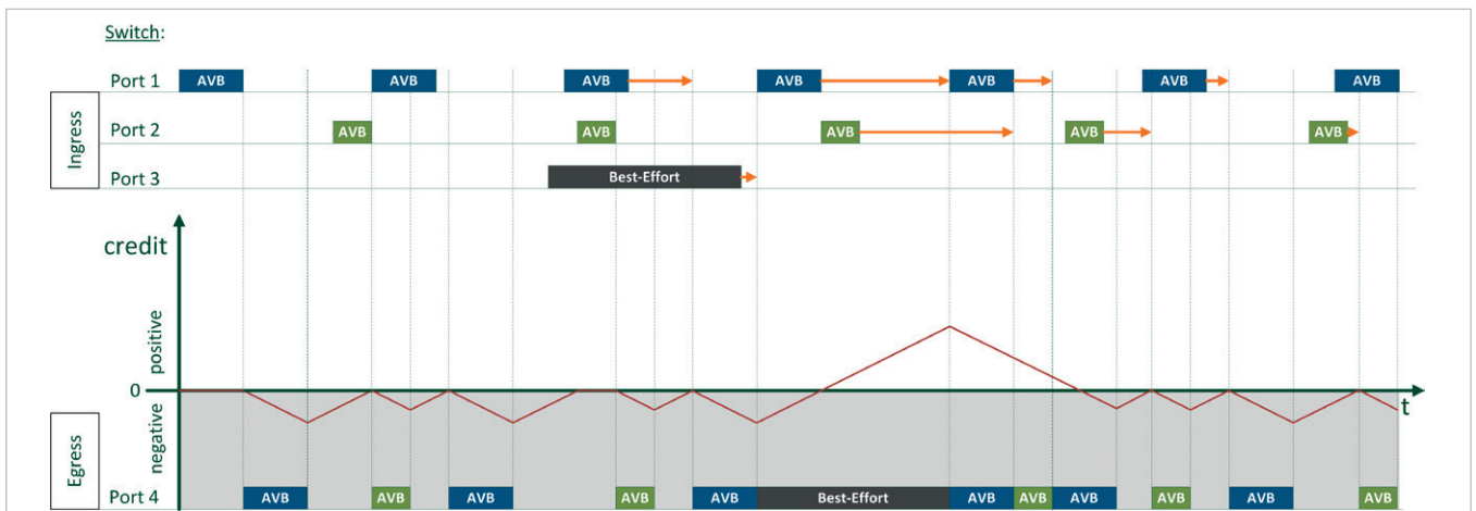
Figure 7: With the Credit-Based Shaper, data streams with reserved bandwidths are handled with higher priority than Best Effort traffic, as long as positive transmission credit is available
