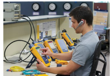
The DSX reduces the time required to fix cabling faults with dedicated diagnostics.
