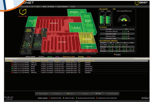
Customizable dashboard view to see real-time values such as alarms, KPIs, PUE and more
