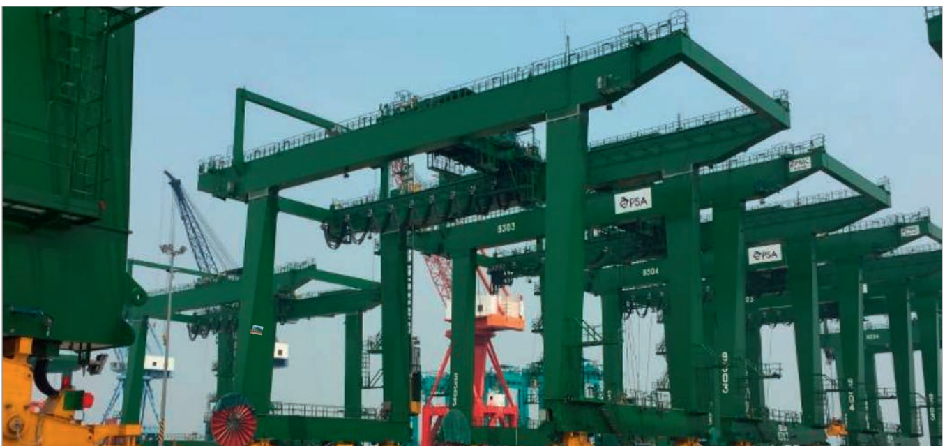
Fully automated Rubber Tired Gantry (RTG) cranes that make container handling safer, more productive and more reliable
