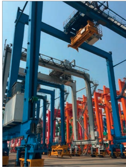
A Rubber Tired Gantry (RTG) crane can move up to 40 containers per hour
